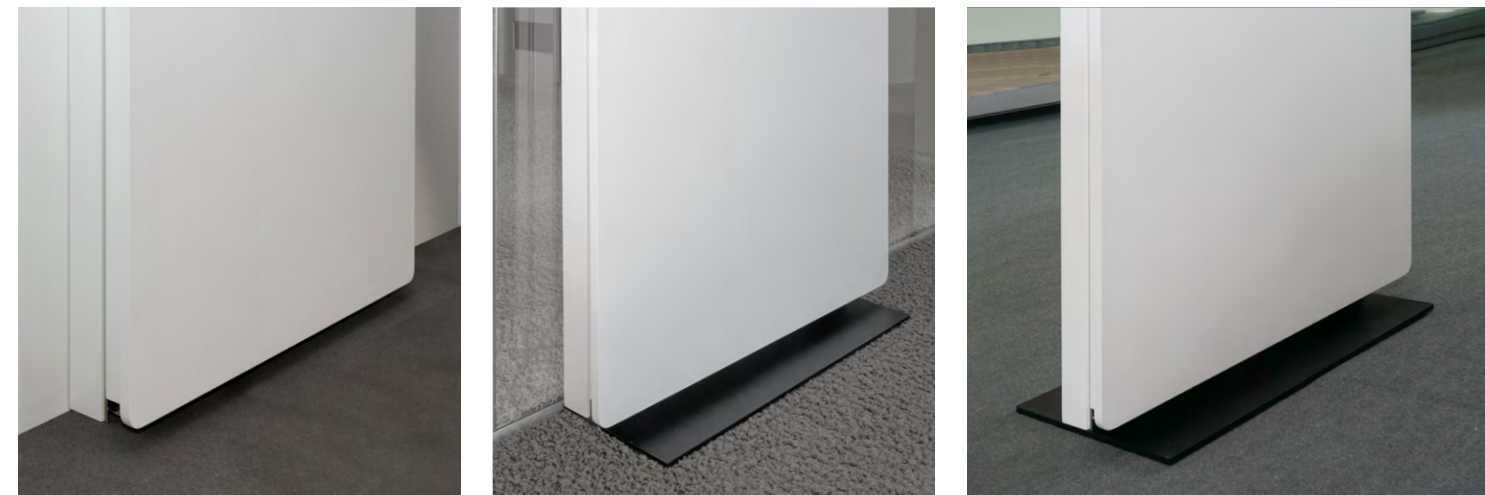
The W6 base module provides load transfer for the displays. Simple wall-mounting is sufficient – also on drywalls without need for elaborate reinforcement! An optional L-foot eliminates the need for wall-mounting, for example in front of a glass wall. An optional T-foot allows free positioning in a space.
